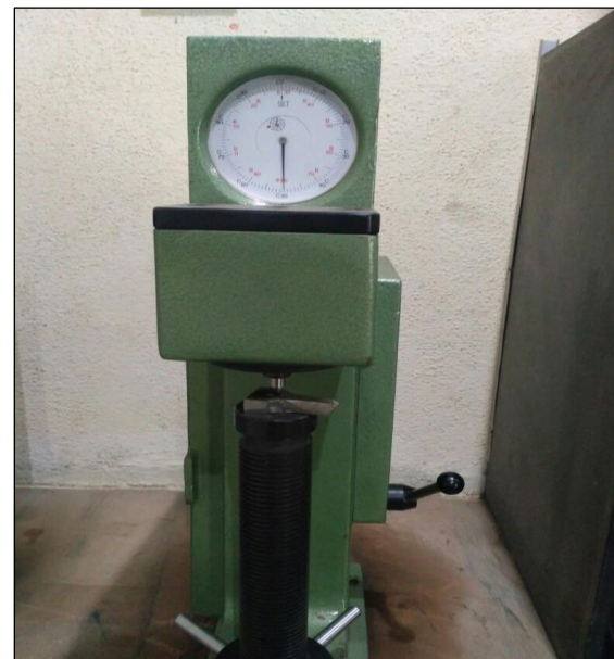
Fig. 3: Rockwell Hardness Tester.
