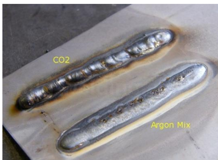
Fig. 2: Part Welded with Argon and Argon + CO 2 Shielding Gas.
