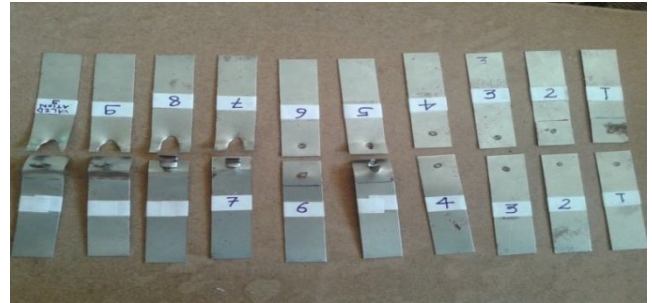
Fig. 5. Specimen failure after Tensile Testing
