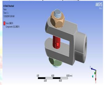
Fig 3.2: ANSYs analysis of screw nut fork assembly (Loading)
