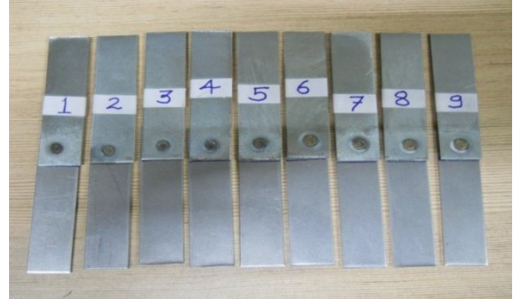
Fig. 3. Test Specimen after spot welding for Ultrasonic and Tensile Testing
