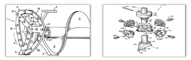
Figure 4. Reuleaux type drill cutter [5] Figure 5. Disassembled type drill cutter [6]
