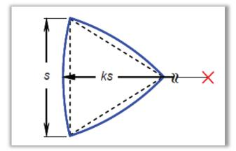
Figure 16 Construction of modified cam geometry of reuleaux triangle
