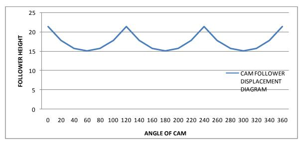
Figure 18.Cam –follower displacement diagram of modified cam.
