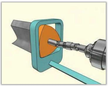
Figure 3 Square hole drilling operation
