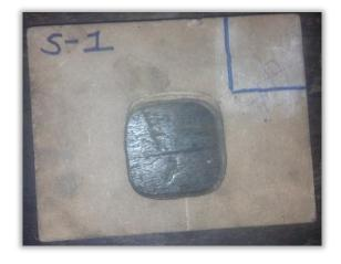
Figure 11. Square hole with existing cam geometry
