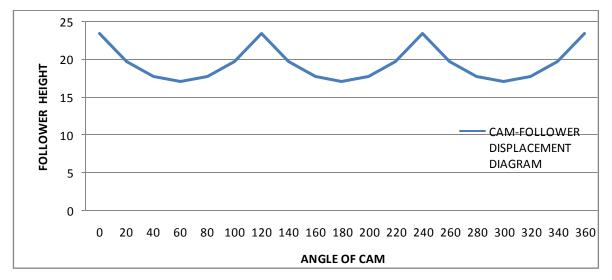
*Figure 17.Cam –follower displacement diagram of existing cam.*
