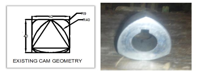
Figure 8. AutoCAD drawing of existing cam geometry Figure 9. Actual existing cam geometry
