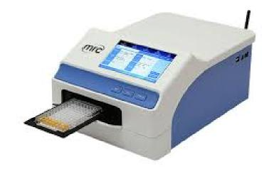
The basic principle of absorbance measurement involves the absorption of light by molecules in the sample. The microplate reader shines a beam of light through the samples in the microplate, and the amount of light absorbed by the sample is measured by a detector. The amount of light absorbed is proportional to the concentration of the molecules in the sample, allowing the microplate reader to measure the concentration of the sample.
