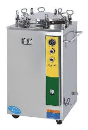
Used for sterilizing equipment and media by subjecting them to high pressure and temperature. The principle of an autoclave is based on the combination of two basic processes: moist heat and high pressure.
