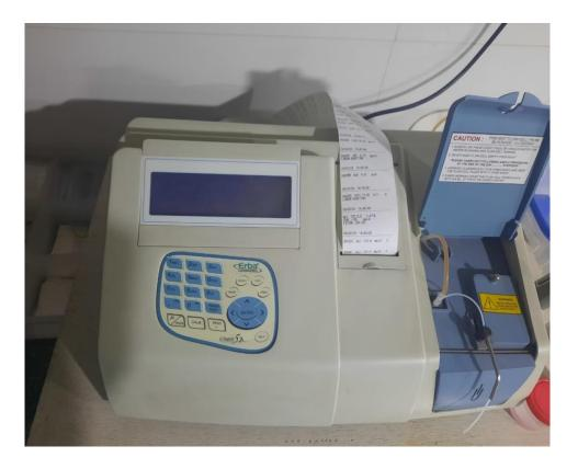
The Clinical Biochemistry Analyzer is an instrument that uses the pale yellow supernatant portion (serum) of centrifuged blood sample or a urine sample, and induces reactions using reagents to measure various components, such as sugar, cholesterol, protein, enzyme, etc.
