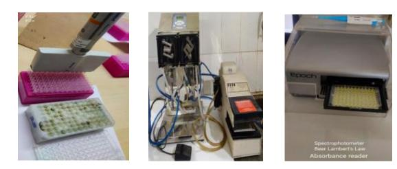
Figure-1: Sample addition (Multichannel Pipette) Figure-2: ELISA Microplate Washer Figure-3: ELISA Microplate Reader with 450/620 nm Filter
