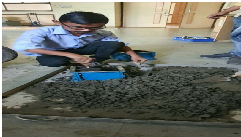
Fig – 4.6 Mould Filling Process
