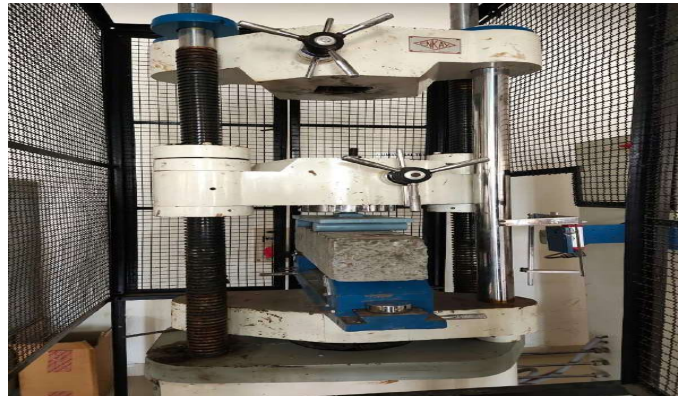
Fig – 4.2 Flexural Strength
