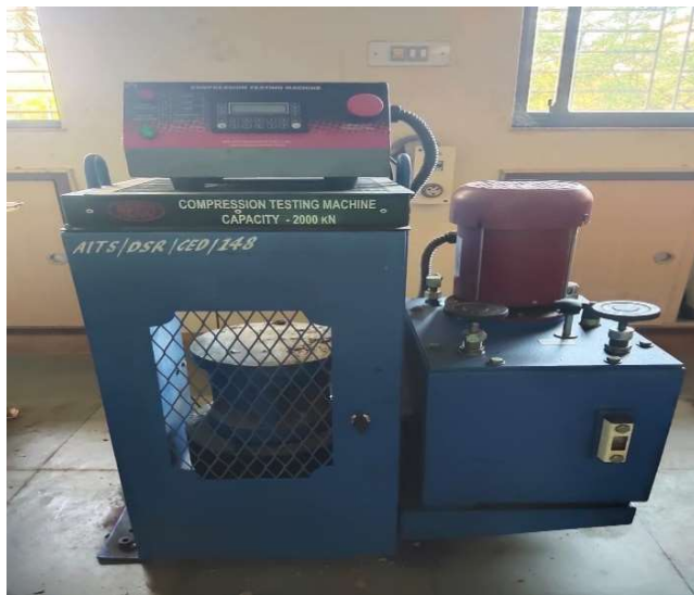
Fig– 4.1 Compressive Strength Test
