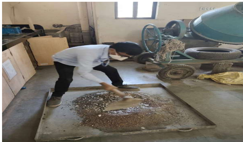
Fig – 4.4 Marble Add and Mixing Process
