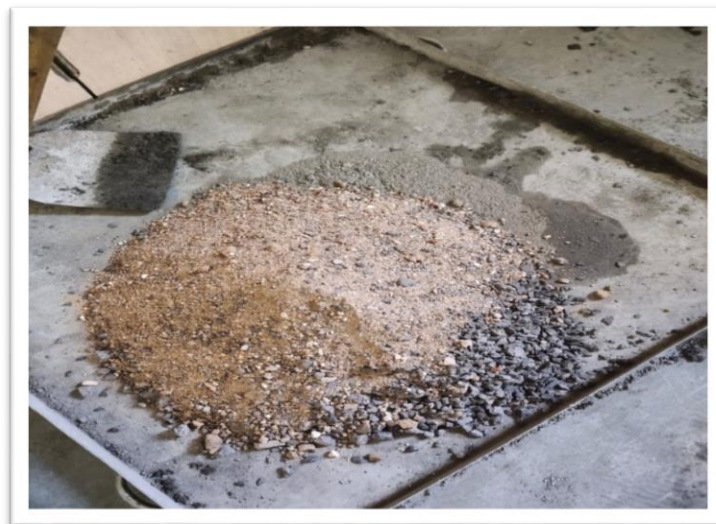
Figure4.1 Dry mixing material
