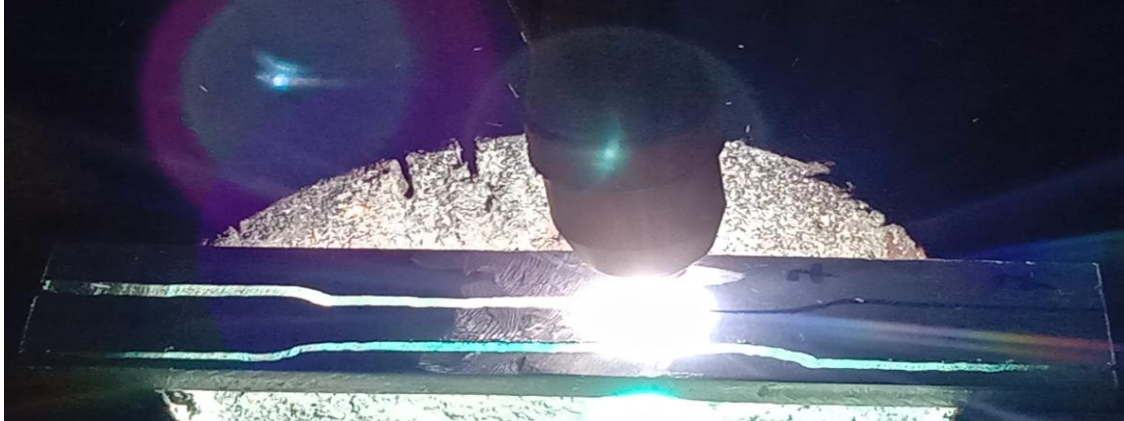
Fig 6.16 – Tensile test specimen preparation using plasma cutting
