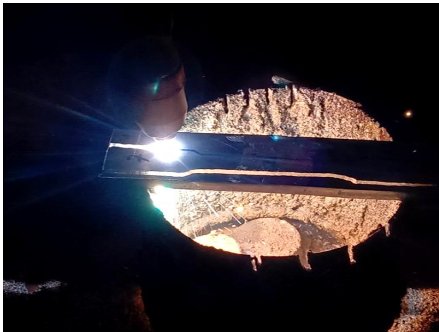
Fig 7.11.2 Plasma cutting of tensile specimen
