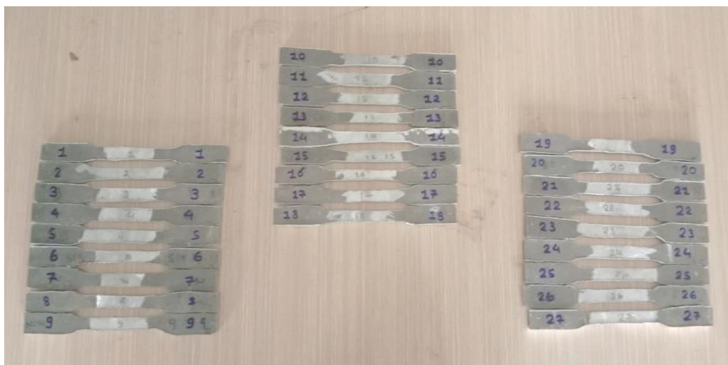
Fig 7.11.4 Tensile specimen before testing
