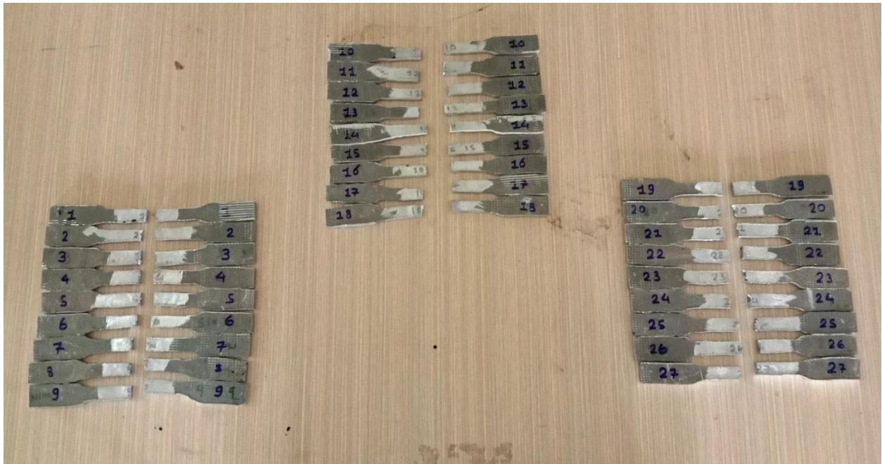
Fig 7.11.5 Tensile specimen after testing
