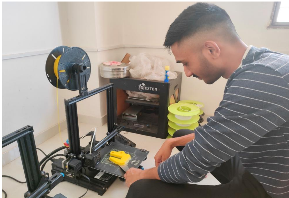
Figure 5.5 Remove C type Hook after manufactured
