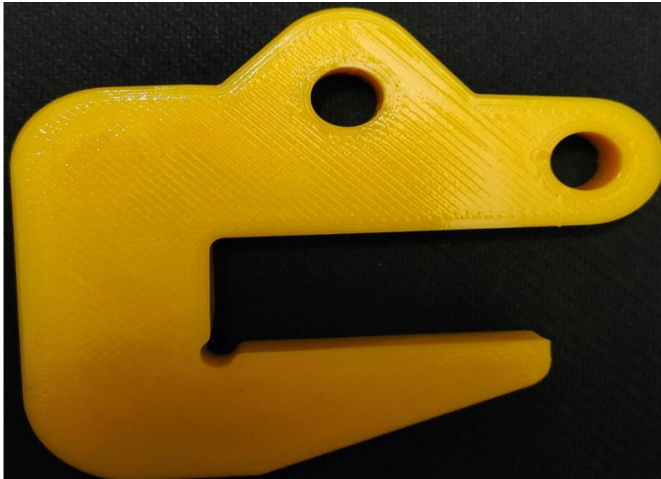
Figure 5.8 After apply Heat Gun on C type Hook
