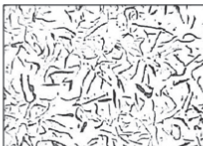
Fig. 2. Image of microstructure at different depths from interface and processed images: a – at 0.5 mm depth from surface and processed image; b – at 1.0 mm depth from surface and processed image; c – at 1.5 mm depth from surface and processed image; d – at 2.0 mm depth from surface and processed image; e – at 2.5 mm depth from surface and processed image; f – at 3.0 mm depth from surface and processed image; g – at 3.5 mm depth from surface and processed image
