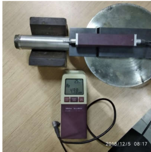
Fig. 4. Surface roughness testing at 0°
