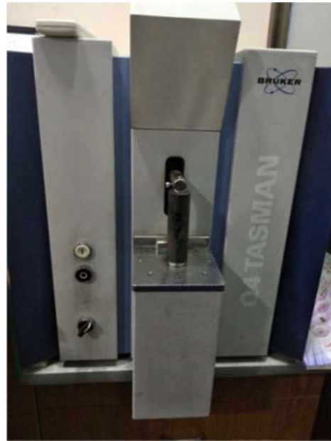
Fig. 2. Chemical Analysis by optical Emission Spectrometer
