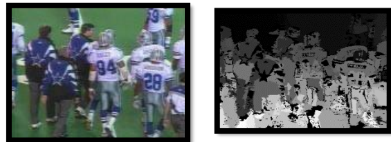
Fig.1: Football image (left) and segmentation into regions (right). Each region defines is a set of connected pixels having same color.
