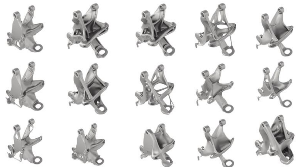
Figure 5 Seat Bracket output of Generative Design
