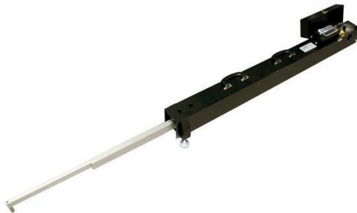
Figure 2: Benkelman Beam Deflection Equipment
