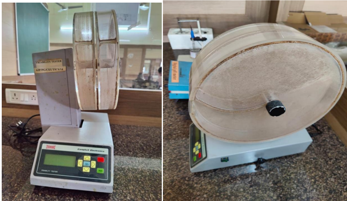
Figure no: 15 Friability Testing Machine
