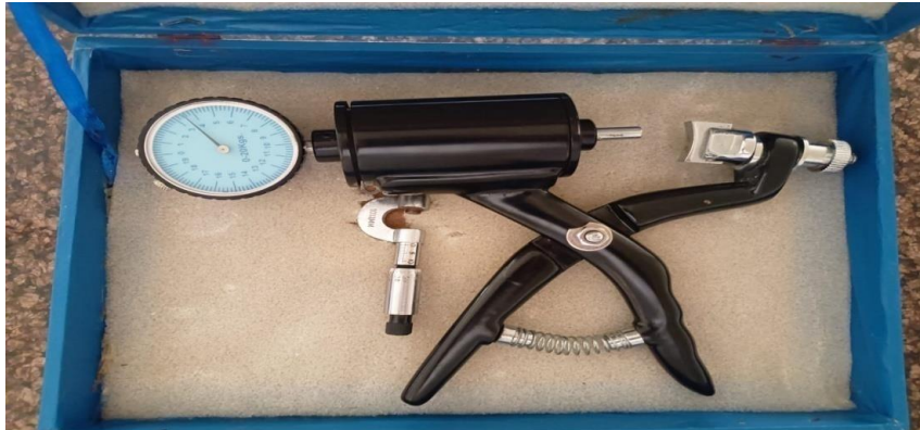
Figure no: 13 Pfizer Hardness Tester
