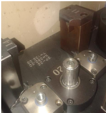
Fig. 13. Collet without Component
