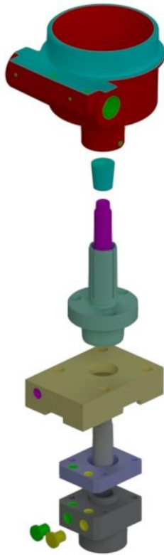
Fig. 10. Exploded Collet-Assembly with Hydraulic cylinder
