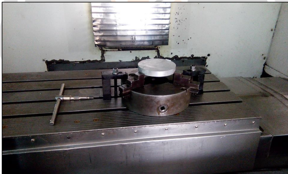
Fig- 8 Setup for machining holes on VMC
