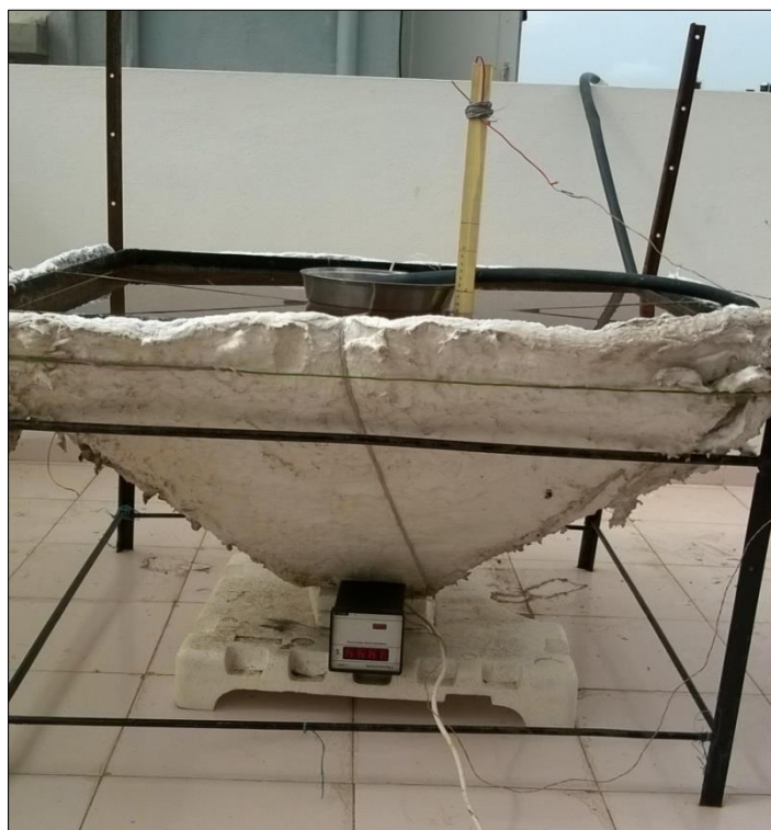
Fig. 2: Photograph of a Salt Gradient Solar Pond.
