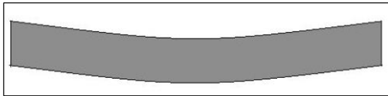
Fig. 7: Distorted Block after Welding.
