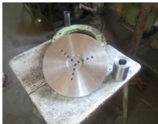
Fig. 4. Disk type Flywheel with stroke adjuster hole. (Real photo)
