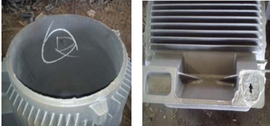
Figure 1 Shrinkage porosity defect in present casting component (see online version for colours)
