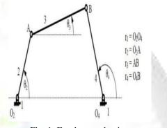
Fig. 1: Fourbar mechanism
