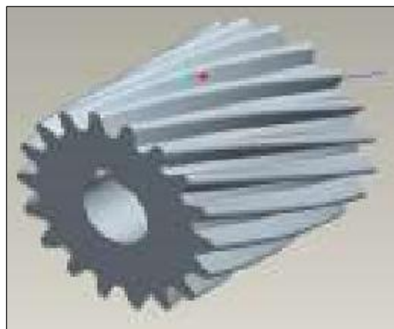
Fig. 8: Solid Model of Helical Gear by Pro-E.
