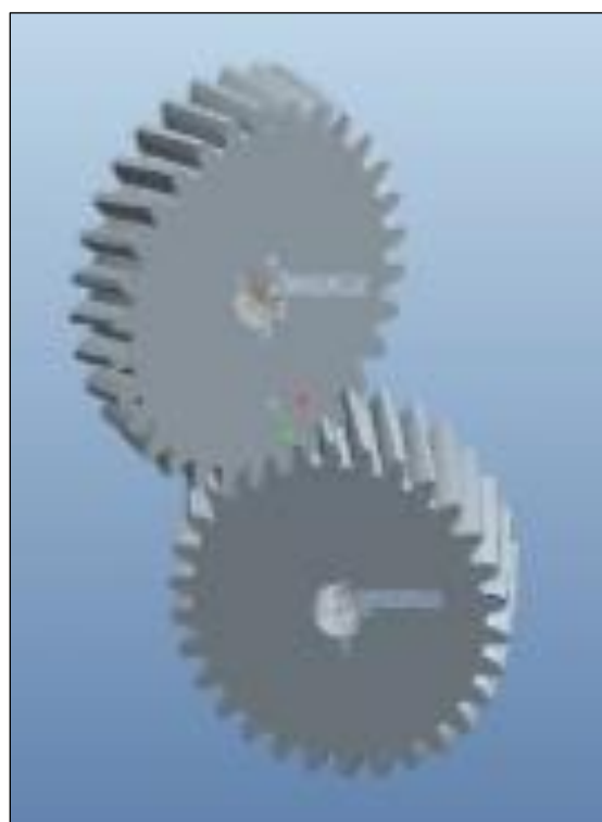
Fig. 4: Modeling of Crossed Helical Gear in Pro/E.
