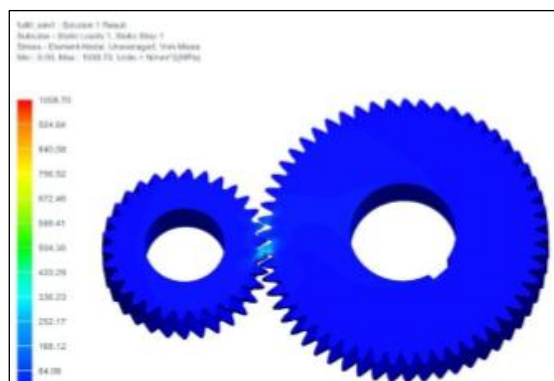
Fig. 14: Contact Stress of the Helical Gear Pair.
