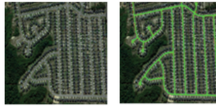
Figure 8. Road are extraction using CasNet Cheng et al. [2017] (a) Sample Image (b) Road Area Extraction
