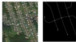
Figure 7. Rasha model for high resolution satellite images Alshehhi et al. [2017] (a) Input image (b) road network and centerline
