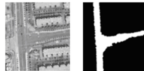
Figure 3. Road detection by Gang Xu algorithm Xu et al. [2009] (a) Test image (b) detected road surface
