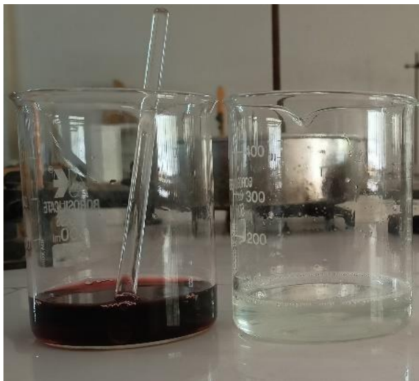
Fig. 5 Mixture of four solution stirred for 30 minutes of lanthanum nitrate + cobalt nitrate + copper nitrate and citric acid
