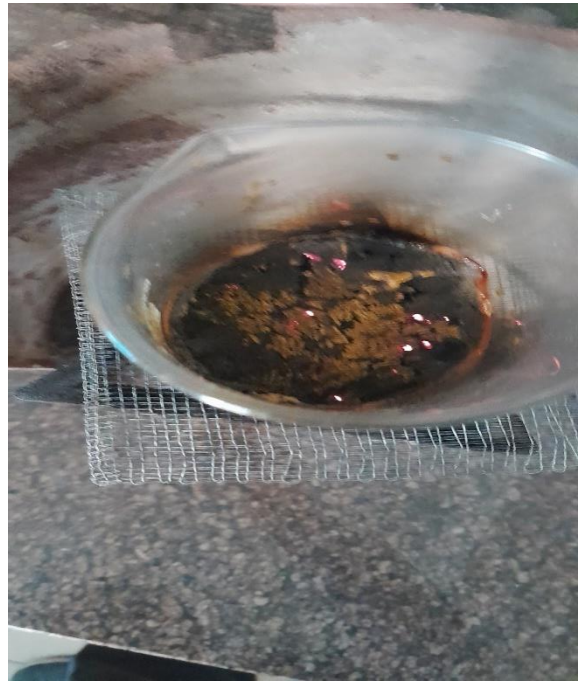
Fig. 14 Drying of gel for solvent removal
