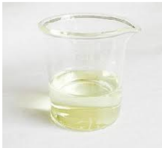
Fig. 10 Mixture of four solution stirred for 30 minutes of lanthanum nitrate + ferric nitrate and glycine
