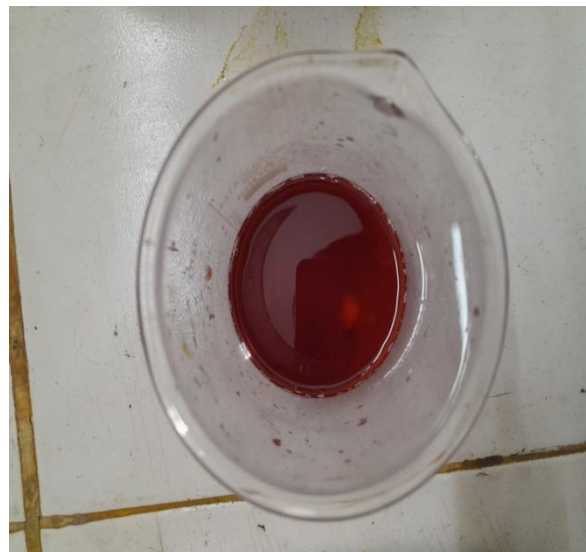
Fig. 5 Mixture of four solution stirred for 30 minutes of lanthanum nitrate + cobalt nitrate + copper nitrate and citric acid
