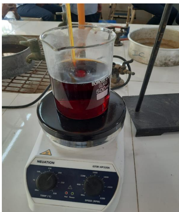
Fig. 11 Mix at 90°C for 2 hours
