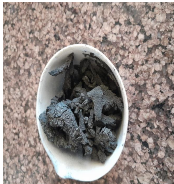
Fig. 8 Calcination in muffle furnace at 800°C for 5 hours (color: black)
