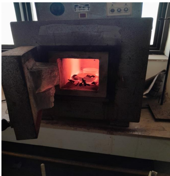
Fig. 8 Calcination in muffle furnace at 800°C for 5 hours (color: black)
