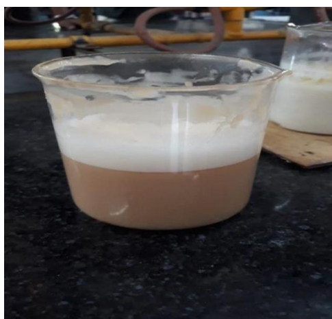
[FIGURE-9 : PRECIPITATION OF CARBOXY METHYL TAMARIND]
