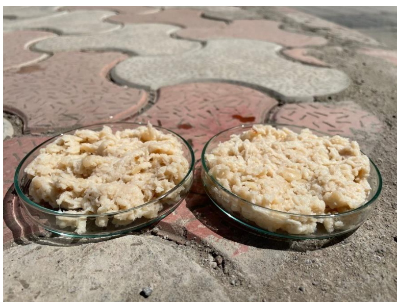
[FIGURE-11 : REMOVING ACCESS OF METHANOL INFRONT OF SUNLIGHT]
