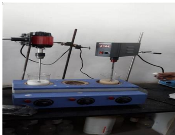
[FIGURE-8 : GRADUAL ADDITION OF SODIUM MONOCHLORO ACETATE (SMCA)]
