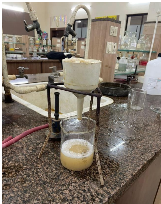
[FIGURE-10 : FILTERATION AND WASH OF 80% METHANOL]
