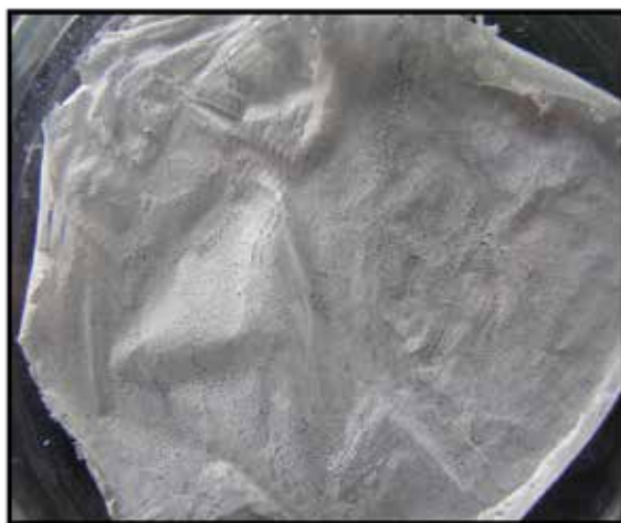
Fig. 5 Crude film of bioplastic (PHB) by Haloarcula sp.1 obtained with optimized conditions
