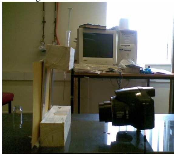
Figure 2. The droplet measurement assembly, with high-speed camera.
